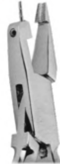
Tweed 786-417 Tweed Loop Forming Pliers. For round or rectangular wires up to 0,56 x 0,7 mm. (.022" x .028"). Replaceable cylindrical beak with three sizes: 1,15 mm. (.045"), 1,50 mm. (.059"), 1,90 mm. (.075"). Concave beak with slight parallel serrations, to keep the wire in proper position
