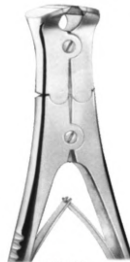
786-444 Wire cutter. For ligature wires and pins. It is strong enough to bend archwire ends after distal cutting. Maximum cutting capacity: wires up to 1,5 mm. (.044"). With tungsten carbide insert.
