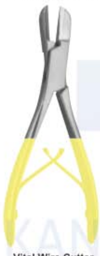
Vital Wire Cutter 10-1202 15cm for hard wires up to 1mm, for soft wires up to 1.5mm
